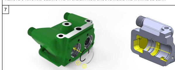
THROUGHLY CLEAN THE SEAT AND ASSEMBLE FIRST THE O-RING AND THEN THE SLIDING PAD. PAY ATENTION TO NOT DAMAGE THEM.
